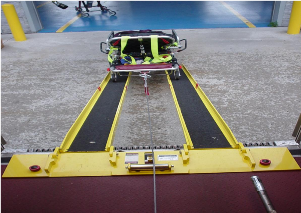
Picture of Winch pulling Bariatric Stretcher into ambulance during loading..
