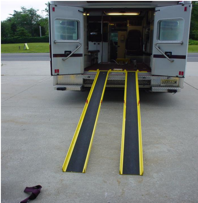
Bariatric Ramps and winch attached to ambulance.
